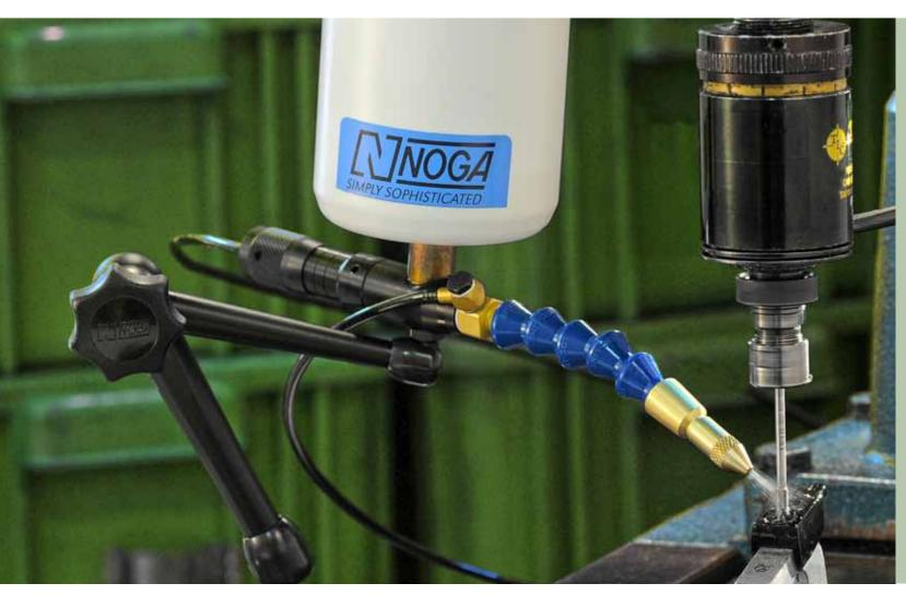
**COBRA 's** drop ejector is designed to accurately shoot small quantities of liquid to distinct targets. An air actuated piston shoots the drops through a flexible hose onto the target.
