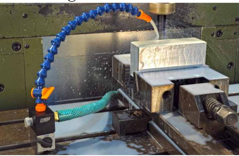
**NOGACOOL** consists of a manifold & Loc-Line® flexible hose with a nozzle on top and a valve at the bottom, assembled on the powerful on/off Popeye magnet.
