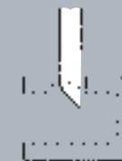
Deburring on internal surface via an opening. Rotate blade 90° from position one, enter opening, rotate again the blade another 90°.
